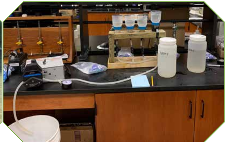
SRBC lab set up to filter eDNA samples collected throughout the lower Susquehanna River Basin to identify range of Northern Snakehead and Blue Catfish. Samples are currently being analyzed by USFWS Genetics Lab in Lamar, PA.
